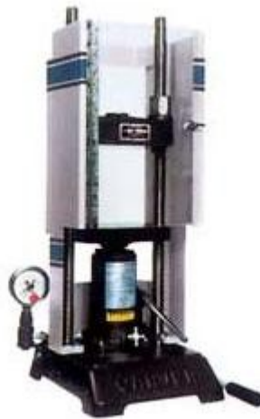
This is a Carver press used to crush the sand during a crush resistance test
